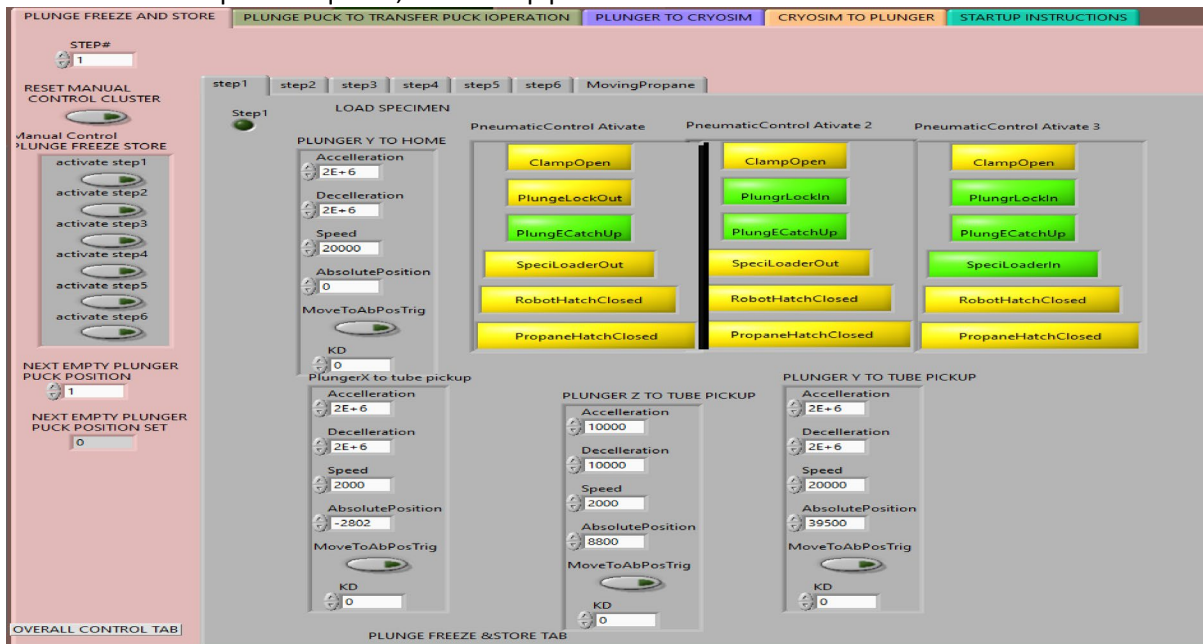
Robotic freezing control panel, use this sequencer when testing warm and for specimen freezing
